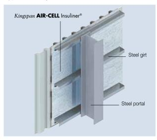
Figure 5 Warehouse wall installation
