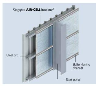
Figure 7 Warehouse wall retrofit installation
