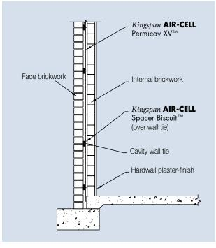
Figure 2 Side elevation of *Kingspan* **AIR-CELL** Permicav XV<sup>™</sup> in double brick cavity wall
