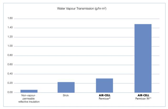
Figure 6 Water vapour transmission comparison.
