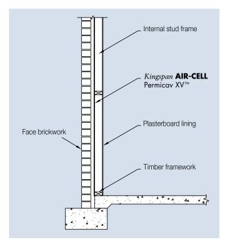
Figure 4 Side elevation of Kingspan **AIR-CELL** Permicav XV<sup>TM</sup> in brick veneer wall
