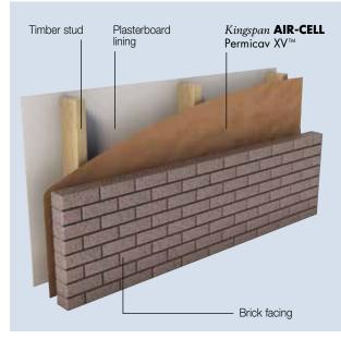
Figure 3 Brick veneer wall installation
