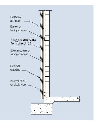
Figure 2 Side elevation of Kingspan **AIR-CELL** Permishield® 65 in a reverse brick veneer wall
