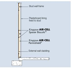
Figure 4 Side elevation of *Kingspan* **AIR-CELL** Permishield<sup>®</sup> on steel-framed wall
