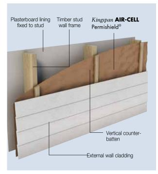
Figure 5 Kingspan **AIR-CELL** Permishield<sup>®</sup> in a timber-framed wall installation using counter-battens
