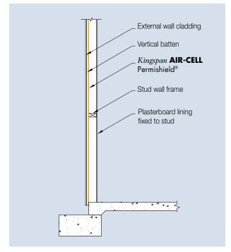
Figure 6 Side elevation of *Kingspan* **AIR-CELL** Permishield<sup>®</sup> on timber-framed wall
