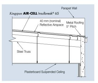
Figure 6 Side elevation of  $\mathit{Kingspan}$  AIR-CELL Insulbreak  $^{\circledast}$  65 in a commercial office
