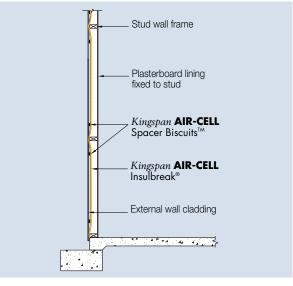
Figure 8 Side elevation of *Kingspan* **AIR-CELL** Insulbreak<sup>®</sup> on steel-framed wall
