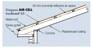
Figure 4 Side elevation of *Kingspan* **AIR-CELL** Insulbreak<sup>®</sup> 65 in a metal roof with a raked ceiling
