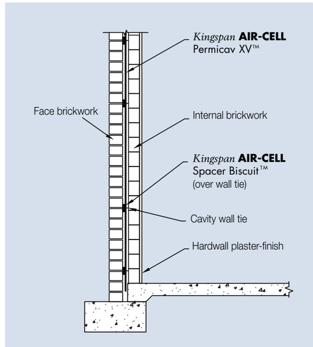
Figure 2 Side elevation of **Kingspan AIR-CELL Permivac XV™** in double brick cavity wall
