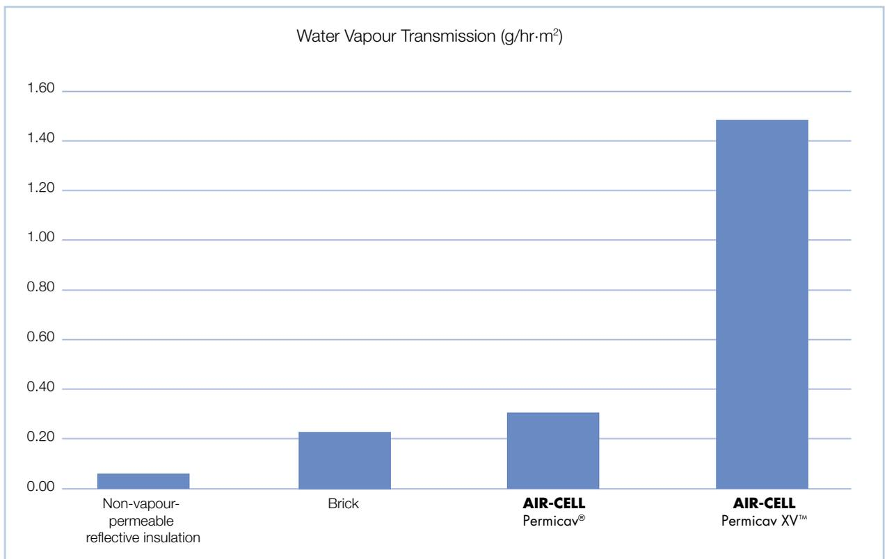
Figure 6 Water vapour transmission comparison.
